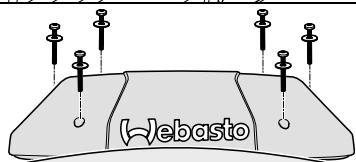
Place the cover on the base plate and tighten with Allen screws and washers.
