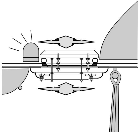
Select the best installation location based on the conditions within and on the driver's cabin with the air distribution plate installed.
