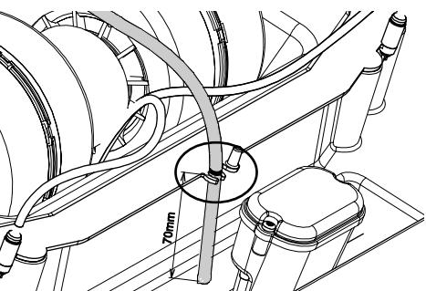
Connect the plug to the base plate. Guide the water hose to the preliminary cooling chamber and insert on the connecting piece.
