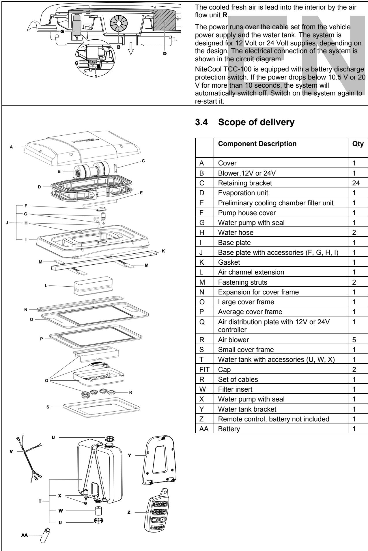
The cooled fresh air is lead into the interior by the air flow unit R.
