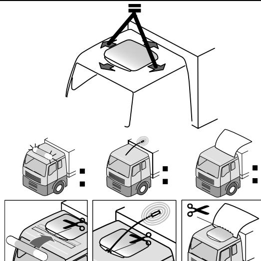
If the base plate will lie on an installed antenna (2) after alignment, cut out the base plate near the front spoiler (1).
