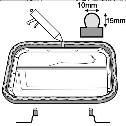
Remove the base plate and put down a sealing strip on the surface of the gasket as well as at the location where the two gasket ends meet.
